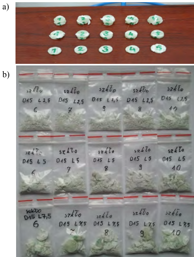
Rys. 11. Failure of specimens: a) under quasi-static loading b) under dynamic loading
